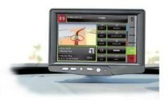
hicles. Combined with a TFT touchscreen, which is provided for quick integration, and a clearly arranged user interface, all components mentioned above can be operated quickly and easily. The application of a transflective TFT display ensures outstanding contrast values and an excellent operability even in case of extreme solar irritation.
